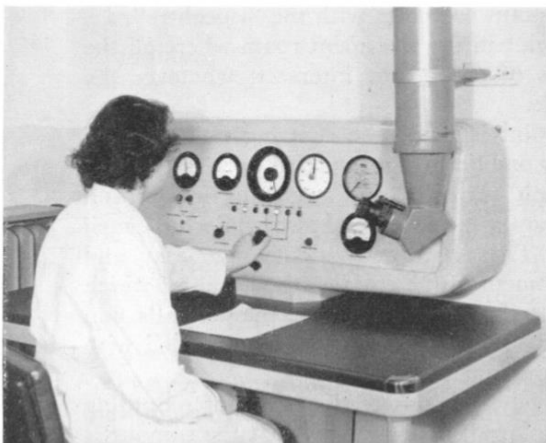
Figure: Control desk for 4MV linac with dose and dose rate meters; and periscope for patient viewing.
