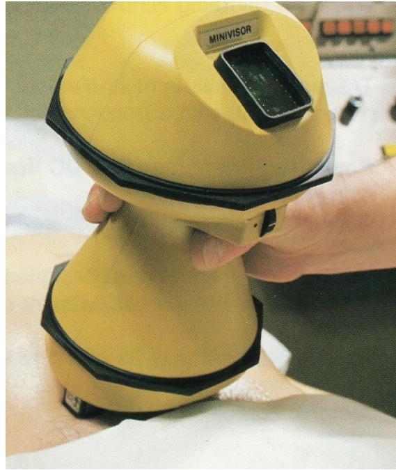
The portable Minivisor, c 1980, with integrated linear array and display
