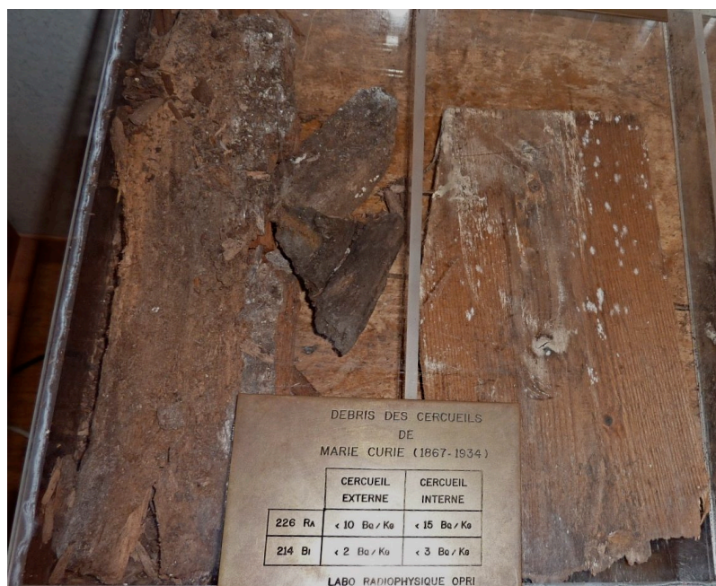
Figure 2: Fragments of the wood coffin for Marie Curie and the results of the OPRI laboratory analyses.
