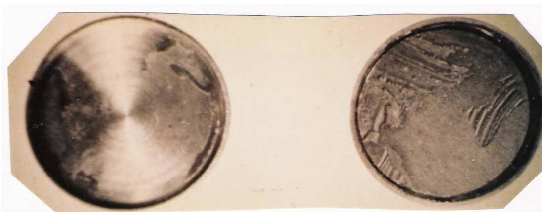
Photograph 3. The suspect coin opened up to show the affixed magnet.
