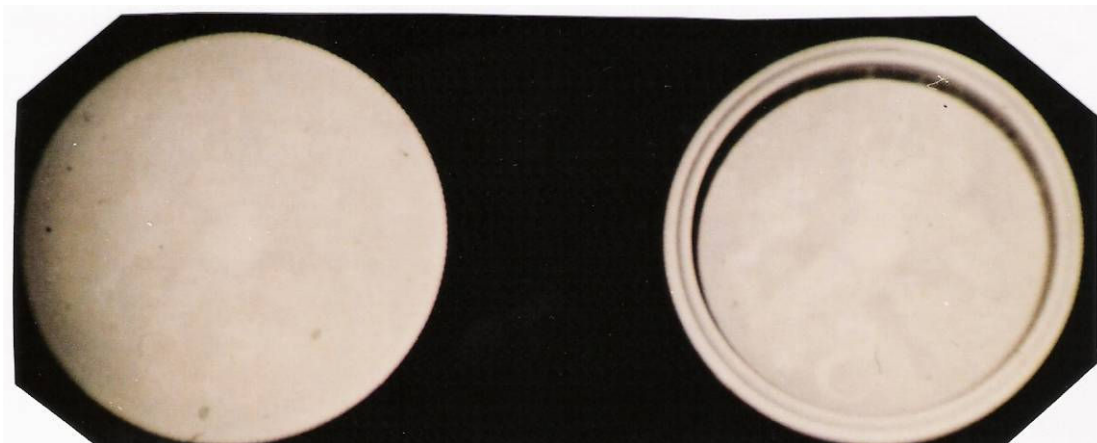
Radiograph of a genuine coin (left) and the suspect coin (right).
